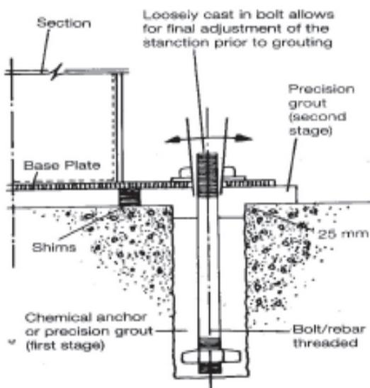
The compressive strength of the grout must exceed 55 N/mm<sup>2</sup> at 7 days and 65 N/mm<sup>2</sup> at 28 days.
