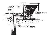
Pouring should be from one side of the void to eliminate any air or presoaked water becoming trapped under the base plate. It is advisable to pour the grout across the shortest distance of travel. The grout head must be maintained at all times so that a continuous grout front is achieved.
