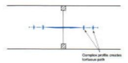
The Supercast range incorporates both of these principles. The products offer a fully continuous 4 bulbed design maintaining both the valve and tortuous path principles. These principles are maintained in the transition from Rearguard profiles in floors to centrally placed profiles in walls.
